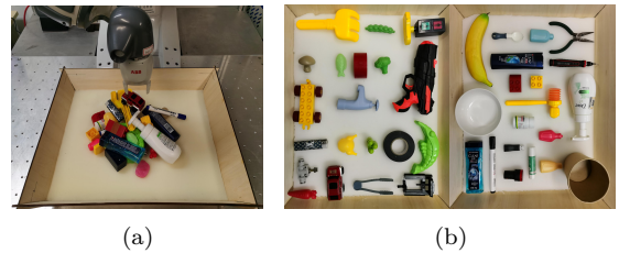
Fig. 7: Real setting of our robotic grasping experiments. (a) Cluttered scene grasping experiment setup with ABB Yumi robotic arm. (b) Objects used in our robotic experiments. Left one shows novel objects which are absent in the training dataset, right one shows similar objects.
